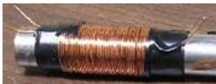
The wire for the third layer is cut to a length of 313 centimetres. Since it will be covering less length along the former, there is no need to build up the ends of the earlier layers. So, simply cover the second winding with tape, and then wind on the third layer, but this time, the coil is wound in a counter-clockwise direction and then the entire coil is covered in tape to protect it.
