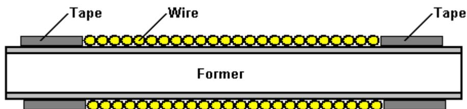
This is so that the second layer of wire will have the same diameter along its entire length. It is probably a good idea to completely cover the first layer of wire with tape to ensure good electrical insulation.
