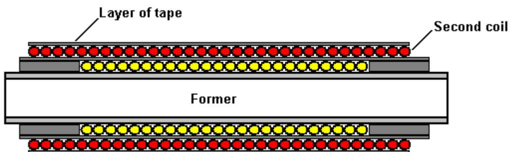
The second wire layer is also wound in a clockwise direction:
